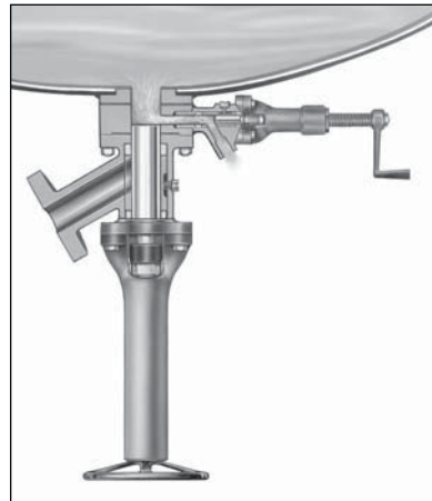
Fig. 2 - Drain Valve Open for Sample
