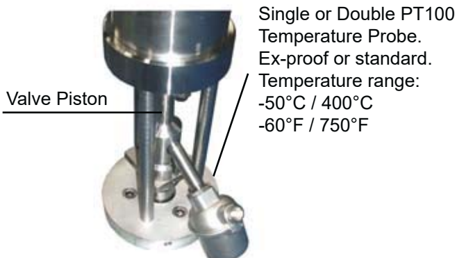
Piston Mounted RTD Sensor
