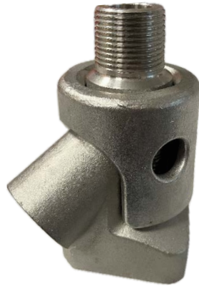
Integral LEPV Jacket on body before welding.
